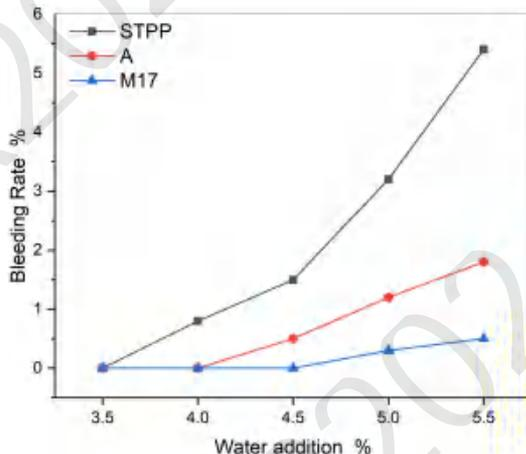
**Test principle:** The bleeding ratio is calculated based on measuring the slurry mass in the receiving tray which released from the castables through the narrow channel when vibrating.
