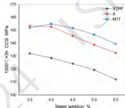
The excessive water addition resulted in the layered bleeding in castables, reducing the long-term strength and bulk density. The sample containing M17 displays the best mechanical properties when subjected to the same degree of water addition.
