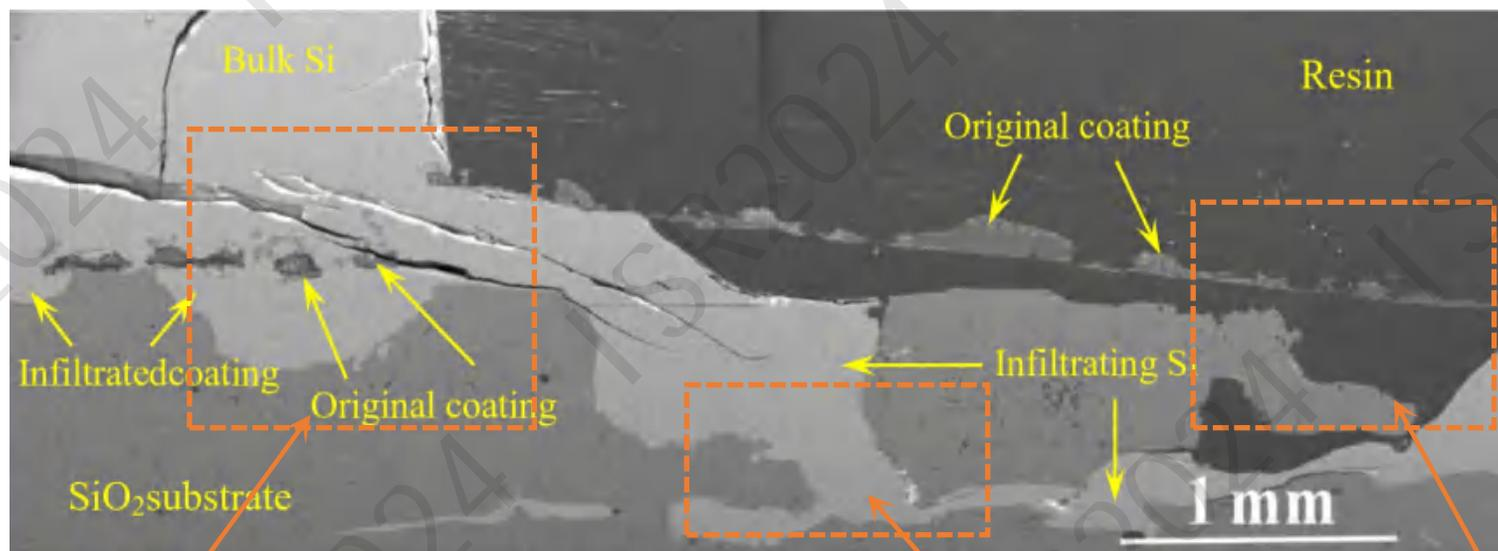
*infiltrated coating of molten Si*
