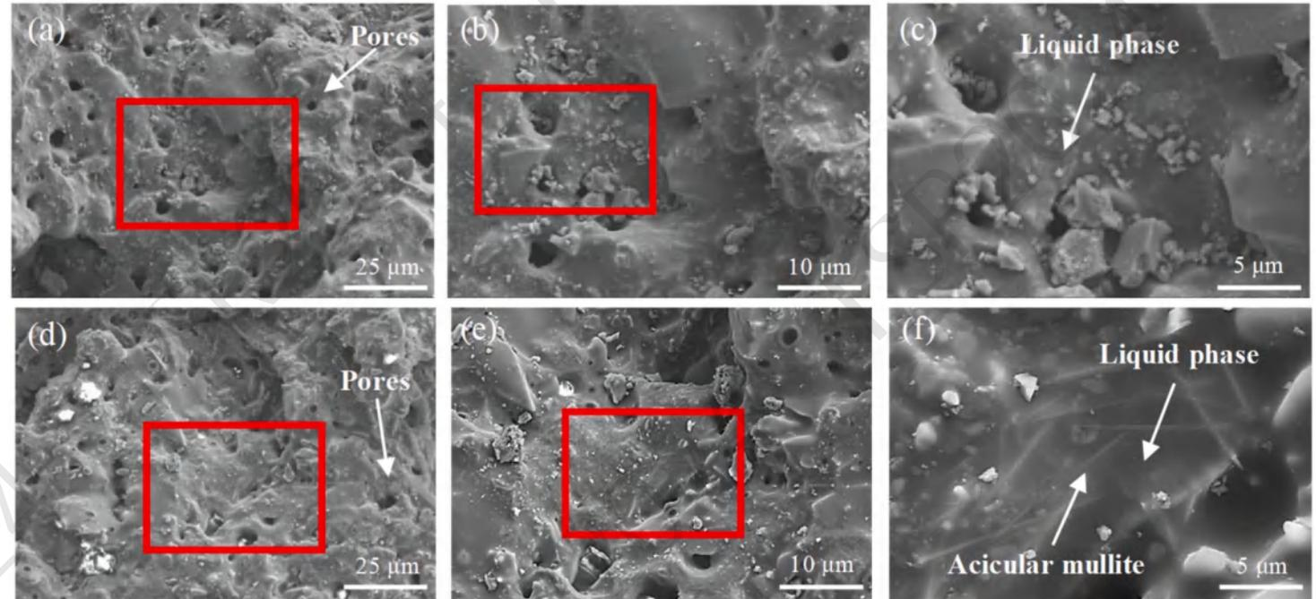
Fig. 3.4 SEM images of the samples after HMOR test: (a-c)SA0, (d-f) SA6
