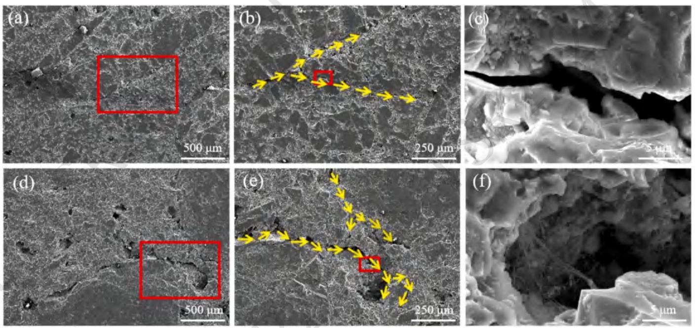
图3.7 SEM images of the samples after thermal shock: (a-c) SA0, (d-f) SA6
