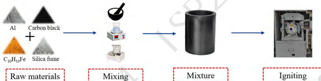
Fig. 2.1 Preparation of composite powder
