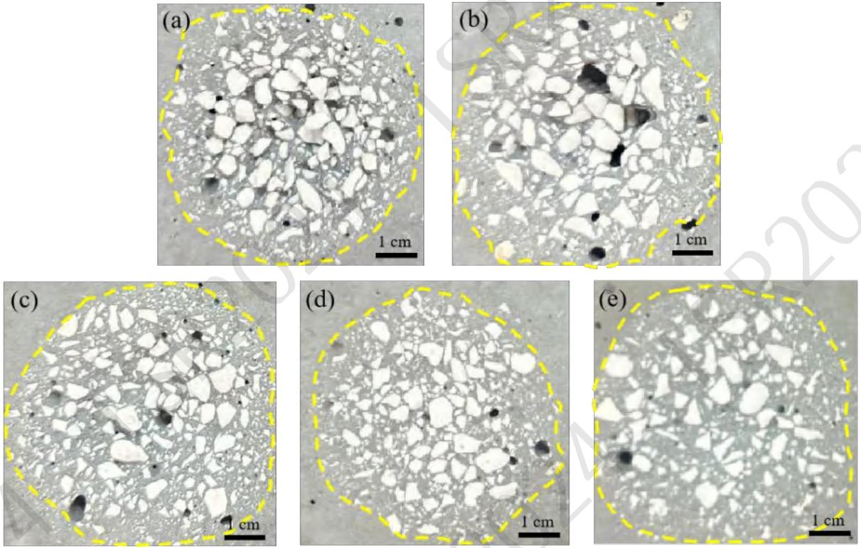
图3.8 Appearance of samples after high temperature wear test: (a) SA0, (b) SA2, (c) SA4, (d) SA6, and (e) SA8
