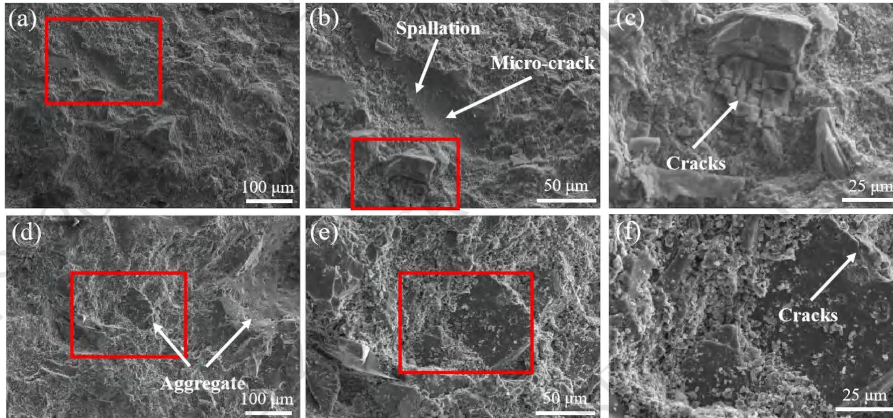
Fig. 3.10 SEM images of samples after high-temperature wear test: (a-c) SA0, (d-f) SA6
