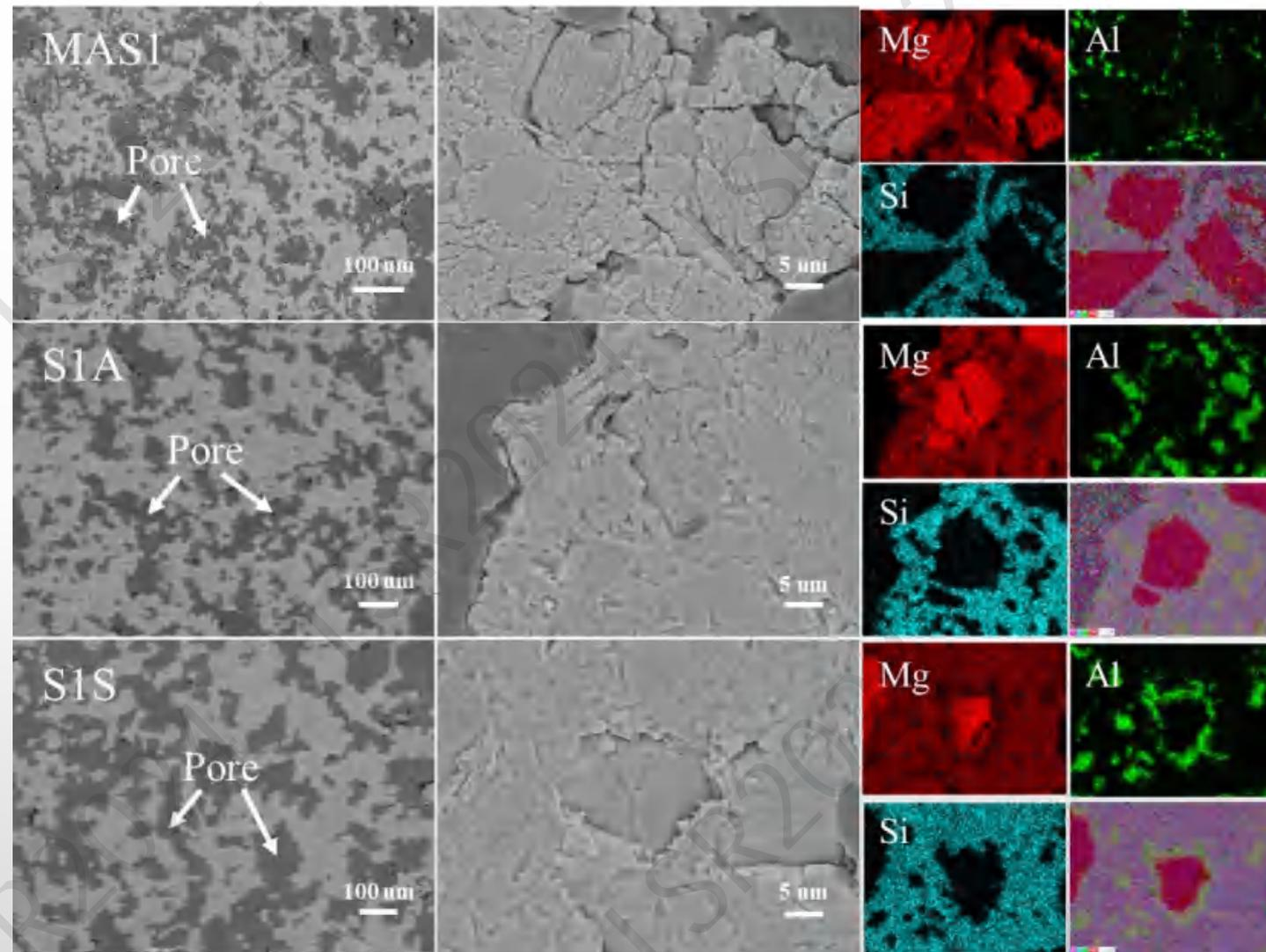
Figure. 9 Microstructure images and EDS mappings of MAS1, S1A and S1S samples sintered at 1600 °C
