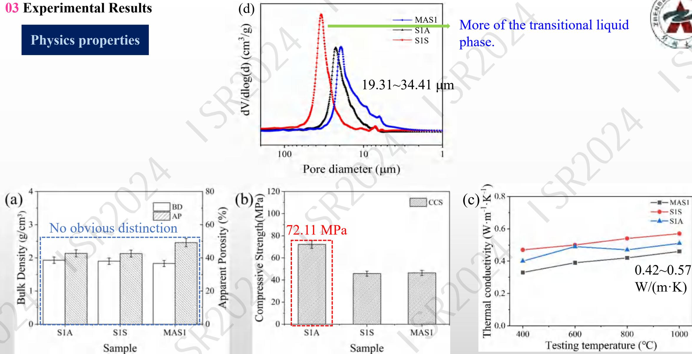
Fig. 10 Physical properties of MAS1, S1A and S1S samples after sintered at 1600 °C : (a) BD and AP, (b) CCS, (c) Thermal conductivity values, (d) Pore size distribution of S1A, S1S and MAS1 samples sintered at 1600 °C
