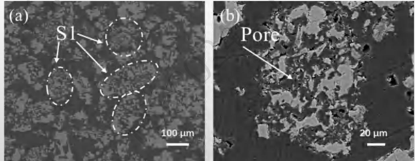
Fig. 6 SEM results of S1 pellet calcined at 1350 °C for 2 h.
