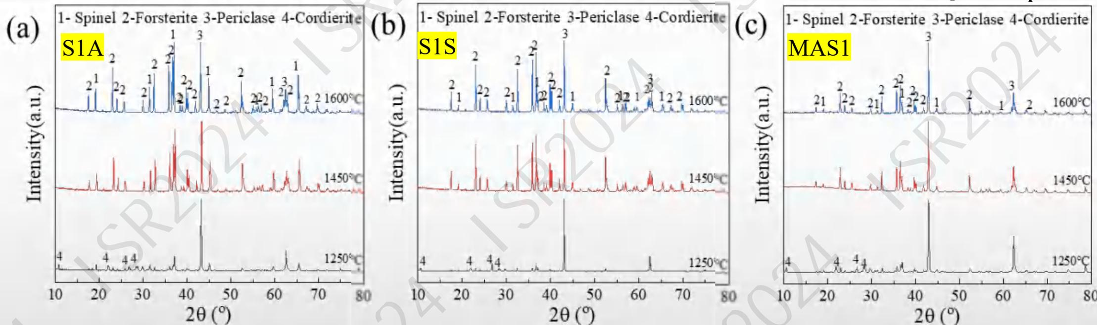
Fig. 7 XRD patterns of samples after sintering at 1250-1600 °C: (a) S1A and (b) S1S (c) MAS1.
