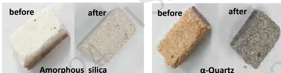
Fig. 10. Specimen before and after hydrogen heat treatment
